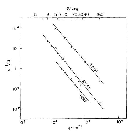
Fig. 1 The inverse  $k^{-1}$  of the first cumulant versus  $q^2$  for three geometries:  $g^{(2)}_{H,V,\perp}(\tau;q_{\perp},0)$ , 0;  $g^{(2)}_{H,V,\parallel}(\tau;0,q_{\parallel})$ ,  $\Delta$ ; and  $g^{(2)}_{H,H,\parallel}(\tau;q_{\perp},q_{\parallel})$ ,  $\Box$ . The identification of  $k/q^2$  with splay, bend or twist distortion of the director field is indicated on the figure.
